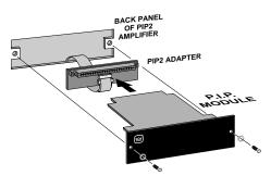
Fig. 3.5 Installation into a PIP2 Amplifier
